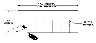
**SEAL ALL PROTRUSIONS ...** Cut a slit around pipes, ductwork, rebar, and wire penetrations to place the initial layer of PERMINATOR. To further protect the concrete slab from external moisture sources, use a piece of PERMINATOR and place a collar around this as well.
